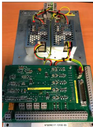
New power supply unit on SCN804
